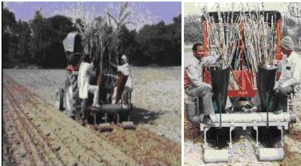
Fig : Improved two row sugarcane cutter planter in operation
