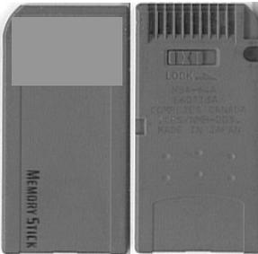
**Memory Stick:** A Memory Stick is an IC (Integrated Circuit) which is stored in a compact and rugged plastic enclosure.
